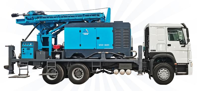
The MWT-350 vehicle-mounted water well drilling rig uses a new SINO HOWO truck chassis and is equipped with a 25 bar two-stage compression high-pressure air compressor. Its lifting force can reach 22 tons, and it can drill water wells with a maximum depth of 350 meters.
